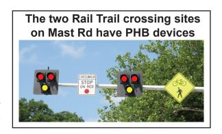
Then both red lights are lit. Traffic must stop. The pedestrian's warning light (on the post at the far side of the road) changes from "DON'T WALK" to "WALK." A count-down display starts its sequence (i.e., 15, 14, 13, etc.) so the pedestrian knows the limits of the safe crossing period.
